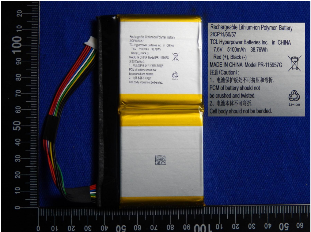
Battery (PR-115957G 7,6V 5100mAh 38,76Wh)
